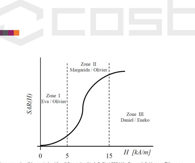
Measurements will be carried out for all 3 samples (No 4, 6, 8) at 300 kHz. For each field zone, T(t) curves will be acquired at 4 different field values and then interpolated. This allows to better take into account the relation  $SAR \sim H^n$ , *n* being different in each zone. For ring test rounds 1 and 2, the ILP was determined assuming n = 2 for all setups.
